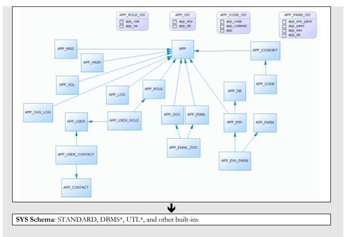
Figure 1: Account Layering within an Oracle Database
